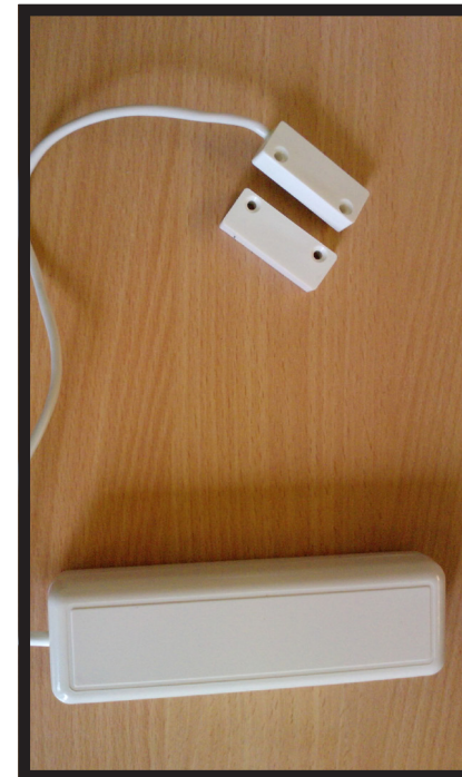
External wireless window sensor (2) © BRE
